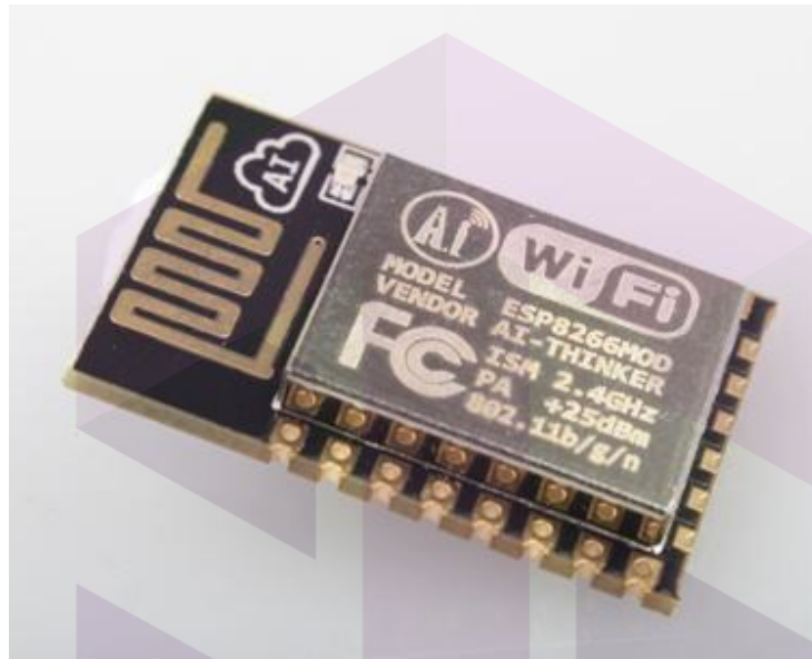
Figure 3 [Module Pin Counts, 22 pin, 16 mm *24 mm *3 mm]
